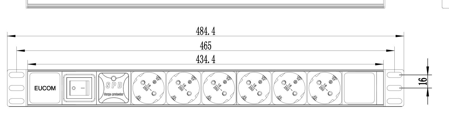
19 inch PDU,1U,Germany type With ON /OFF Switch and Surge Protector Cable: 3G 1.5mm<sup>2</sup>, Cable length, 1.8M
